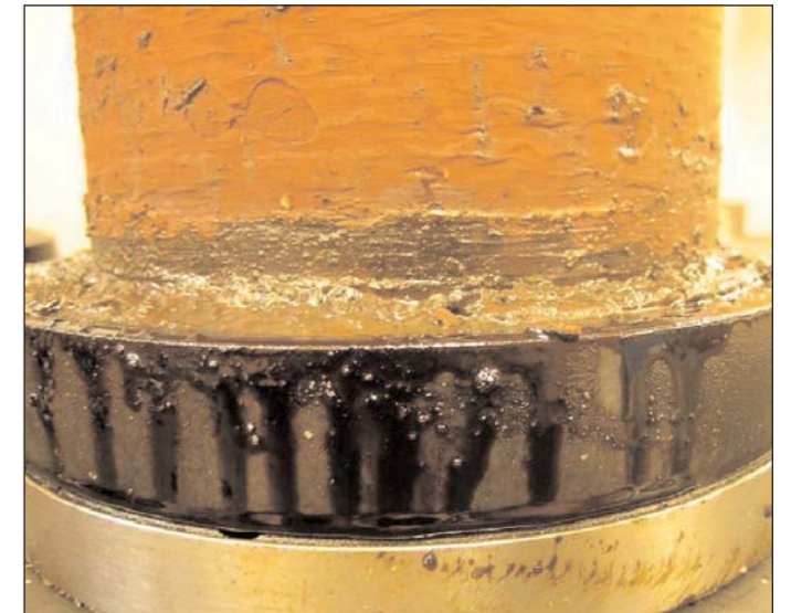
Figure 4 – Typical API682 seal with the Multiple Springs located out of the Process Media.
