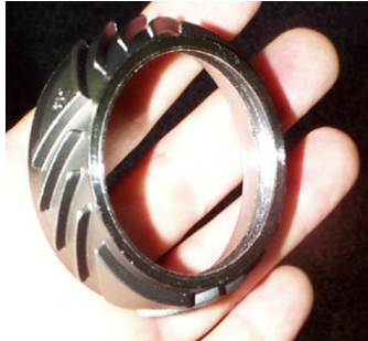
Fig. 16 – Investment Cast Taper Vane Pumping Ring
