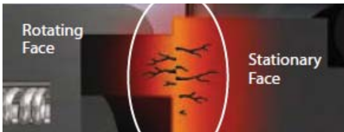
Figure 2 – Mechanical Seal “Poor” Fluid Film
