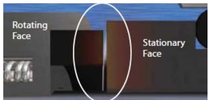
Figure 1 – Mechanical Seal “Good” Fluid Film
